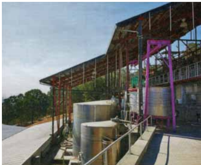
Calera's winery, a gravity-flow operation encompassing seven levels, occupies the site of a former rock-crushing facility. “Calera” comes from the Spanish word for limekiln.
